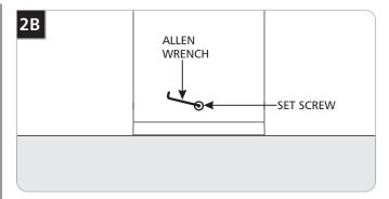
Carefully install the fixture onto the base plate and secure it in place by tightening all set screws.
