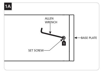
Loosen (Do Not Remove) the set screws on fixture base with the provided Allen wrench and remove the base plate.
